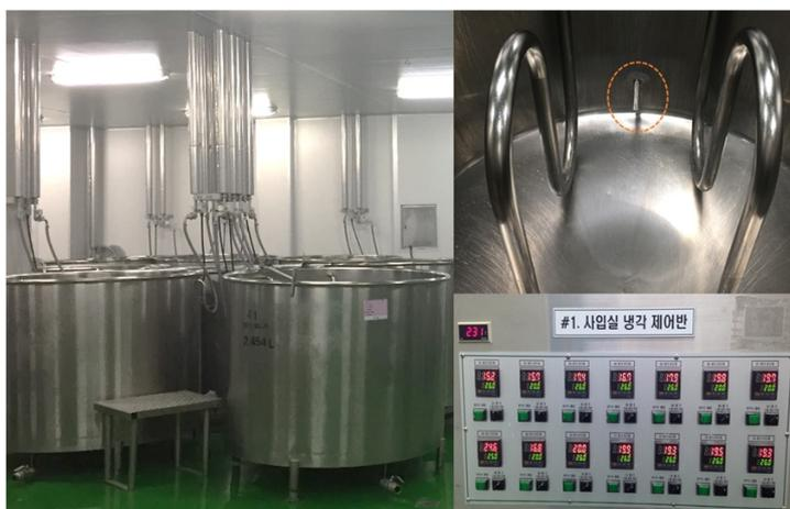
Figure 1. Fermentation tanks and controllers (left), Temperature sensor inside a fermentation tank (upper right), and control panel for controlling temperature of a fermentation tank based on the temperature sensor (lower right)
