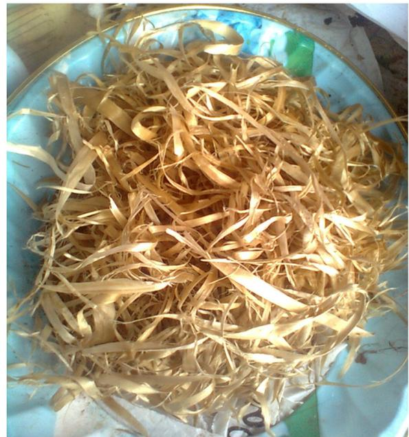
Figure 1. Bamboo sheaths used for pulping.
