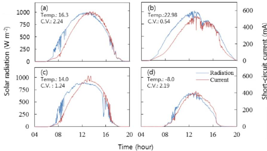
**Figure 3.** Comparison of solar radiation and short-circuit current on (a) April 17, (b) June 20, and (c) October 1 2011 and (d) January 6 2012. Temp. and C.V. denote the daily mean ambient temperature ( $^{\circ}\text{C}$ ) and cloud cover (overcast=10) during sunlight hours.
