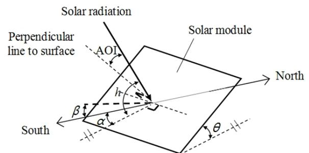
Figure 1. Angular relationships between the AOI and the surface of the solar module ( $h$ : solar altitude angle,  $\alpha$ : surface azimuth angle,  $\beta$ : solar azimuth angle,  $\theta$ : inclination angle of the surface).
